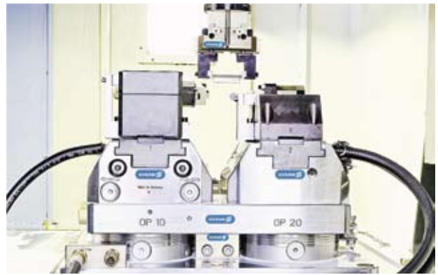
SCHUNK TANDEM plus clamping force blocks are specially designed for the requirements of automated machine loading. In this lean automation solution, they are combined with a SCHUNK VERO-S NSL plus clamping station and loaded via the machine's own axes.
