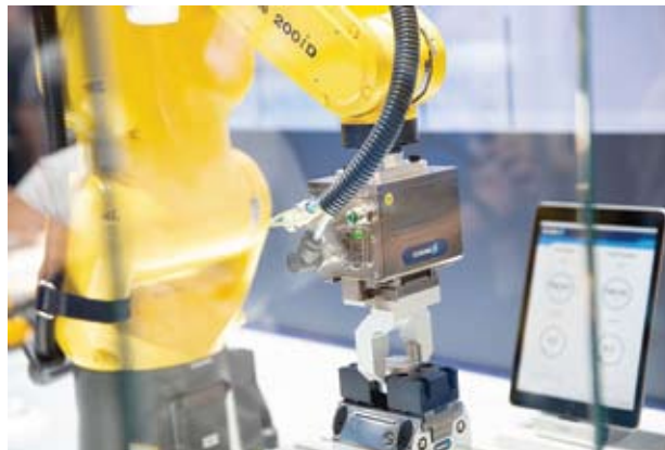
The smart clamping devices and gripping systems from SCHUNK measure, identify, and monitor gripped components and the ongoing production process in real time.
